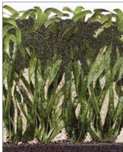
Synthetic turf is actually a complete system of grass fiber, infill and backing, laid over a foundation of earth, sand and/or concrete. Components are fine-tuned to the environmental conditions where a field is being installed.
